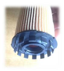
Install a new filter housing "O" ring. Seat filter as shown below into the clean oil filter housing. Lubricate all "O" rings with fresh oil.
