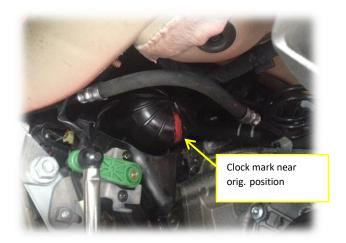
Oil filter housing should be fully seated snug against the base and as it seals on the outside "O" ring.
