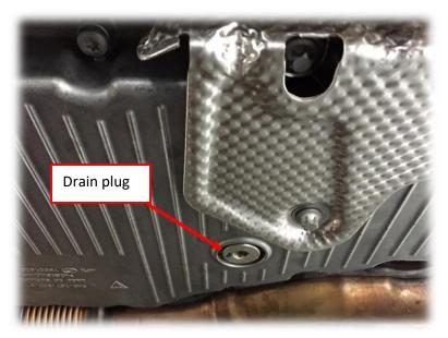
Remove oil drain plug from bottom of engine. Let drain for one hour. Install plug with new crush washer. Torque to 37 ft. lbs. with 8 mm hex key drive.
