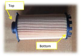
Inside oil filter cartridge. Note center stem or "spud" for locating bottom opening of filter.
