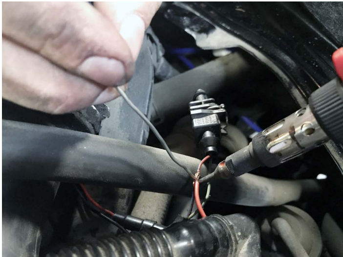
Pictured Left: Securely solder or crimp the power connection
