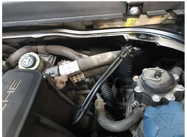
Pictured Right: Find a position of your choosing to mount the valve controller box
