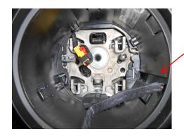
Cable must lay in this slot.
