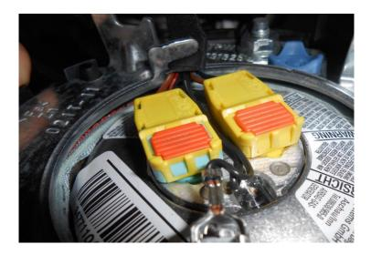
Use the flat bladed screw driver to gently pry up the orange tabs on both connectors. Remove the connectors. Do now worry they are color coded and match the fitting on the airbag. Also remove the metal clip.
