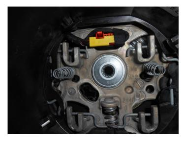
Remove the yellow connector by depressing the red tab and pulling. Now you get to use that new tool. Place the 12 mm Serrated Wrench in the wheel bolt. Use the ½ inch socket to turn the 12mm wrench.
