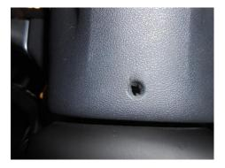
What you are trying to do is push up on a metal bar. This pushes up the teeth that hold the airbag in place
