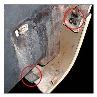
The lower circle shows the lower attachment point (#'s 3/4/6 above). Screw (#3) should be removed to allow the panel freedom to flex.
