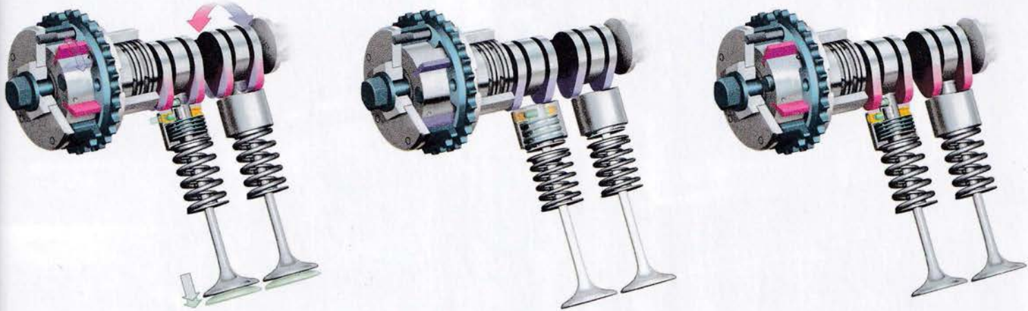
Above VarioCam technology: the valve timing of the intake camshaft can be changed in a fully variable manner using the vane cell adjuster
