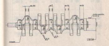
Grind bearing surface for oil seals to dimension 89.8 only if score marks are too deep. In other cases, repolish if required  $R_t$ =0.8...2. Oil bores are rounded to R 0.5 after grinding. Remove sharpe edges with R = 0.2...0.5. Max. permissible radial runout relative to support max. 0.04.
