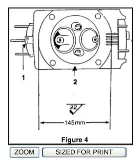
5. Machine 0.10 +/- .02 mm from inner surface (arrow 2 in Figure 4). The diameter of the machined surface must be 145 mm (Figure 4). A surface quality standard of 32 micro-inches must be maintained. Machining should be done with a cutting tool at right angle to the work. The cylinder head surface may only be machined a maximum of 0.20 mm.
