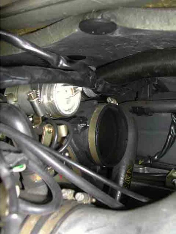
It's also easy to see where the other two connectors were plugged into, on the ISV and just underneath it.
