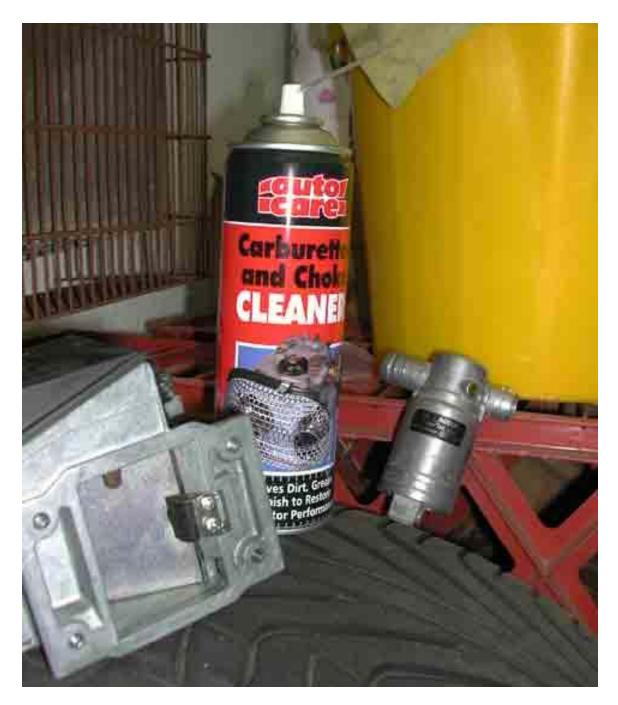
I cleaned the contacts on the ISV and air-flow meter and the contacts on the plugs in the car (note carb cleaner carries warning about using on rubber and plastic, so I used a cloth to avoid spraying those bits) then cleaned the ISV and air-flow meter themselves. You can remove the plastic lid from the air-flow meter (cut the sealant and lift off), and clean the contacts inside, but I decided to leave that for another day if my idle problem isn't cured. Loads of gunk came out of both bits.
