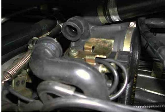
The idle microswitch is the black rectangle with the cable running to it under the long spring;
