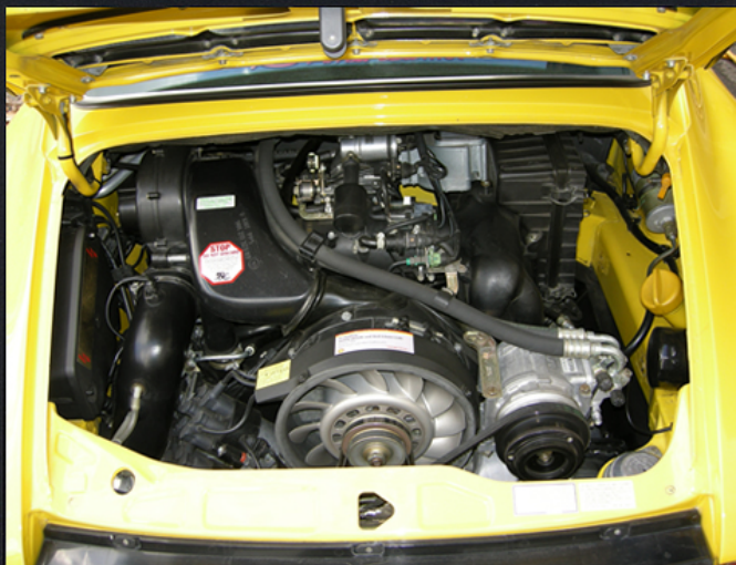
Unlike the European RS, the RS America used the standard 250bhp Carrera 2 engine
