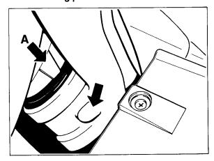
The car ride level height is adjusted on the rear and front axles by turning the adjusting nut on the bottom spring retainers. Use a hook-type wrench or Special Tool VW 637/2 (lever) for this purpose.
