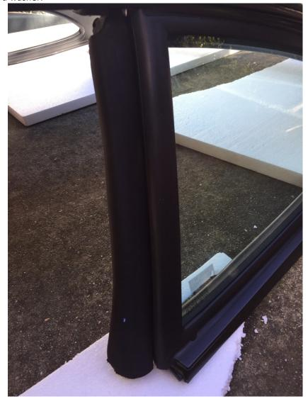
Now you can put the top section in. There are 4 holes where you screw this part directly into the plastic of the hard top. I asked if that was truly the case, and it is. I have not done this yet, but I want to find a better solution (potentially using some of the enclosed metal brackets (top right in the parts picture, in brass) as I haven't found where those go, and I dislike the idea of metal into plastic.
