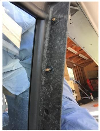
Rear view of the window gasket. The front side has the metal bar sandwiched between the fiberglass and the short part of the window gasket removed from the convertible top (see picture below)
