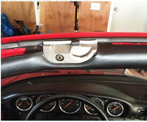
Fix the two male locks inside the hard top using the hex bolts and washers. Be sure to note that LEFT refers to the drivers' side and RIGHT refers to the passenger side, unless you are in the UK. I did have a washer for the top left bolt, just not pictured.
