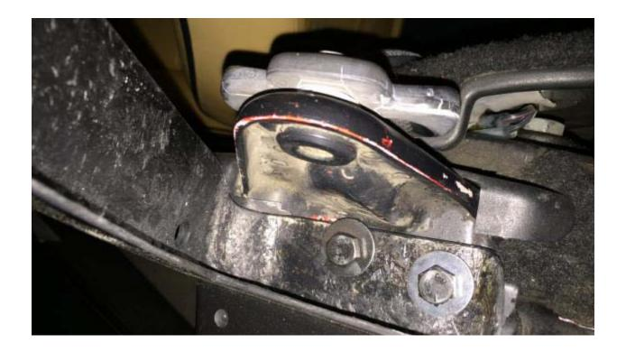
Now you must secure the three rear anchor points. The three "bent" L shape brackets are where these bolts ultimately connect to. In the soft top removal, you may have left the original brackets, which are bolted onto 2 threaded studs that are welded onto the body. Remove those, and place the "bent" L brackets in their place. The one with no angle fits in the center, and the other two match the curvature of the hard top (e.g. the one on the right, passenger, side angles to the right).
