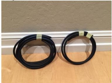
I found that both gaskets go on the farthest possible ridge on the hard top. In the front section, there is a secondary ridge that is closer to the rear of the car, but put it on the outer most edge.
