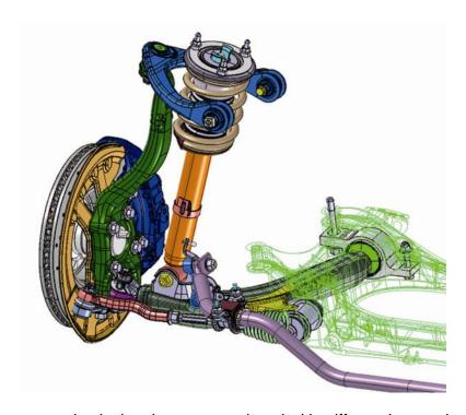
Monotube gas-pressure shock absorbers are employed with stiffer springs and a larger stabilizer bar—all optimized to precisely control body, wheel and suspension motion. The stabilizer bar is hollow to reduce weight. The rubber "bound stoppers" that cushion the compression stroke are unusually long and are invoked early to help control body motions. Ride height has been reduced in both front and rear for a lower center of gravity to minimizes body sway and lateral weight transfer.
