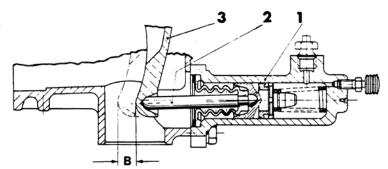
If distance is less than 15 mm there can be no guarantee that clutch disengages fully.
