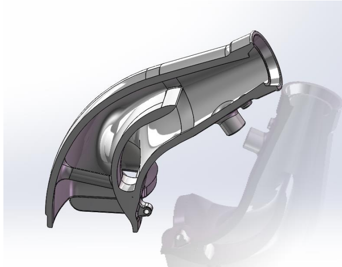
Figure 2.2 Cross-section of a Dual Plenum Manifold
