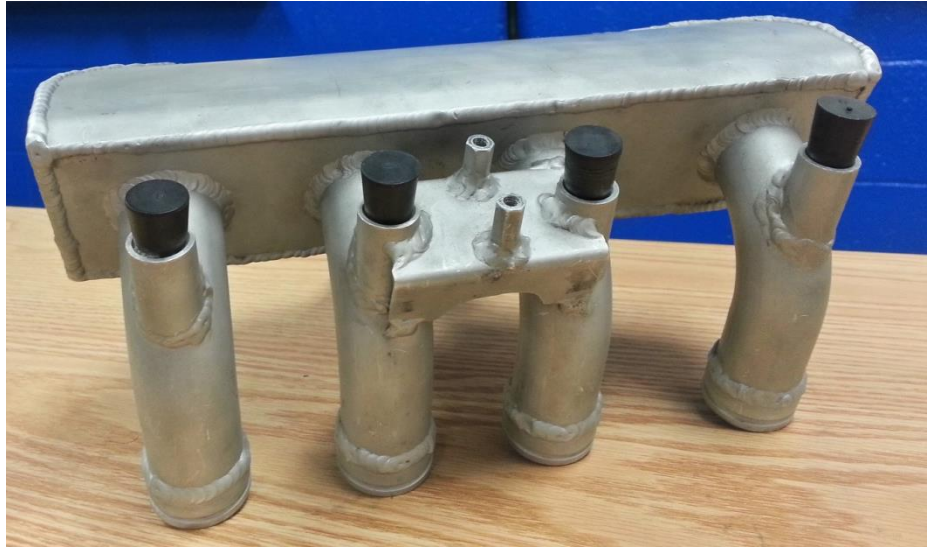
Figure 2.3 F06 UTA FSAE Dual Volume Plenum Intake
