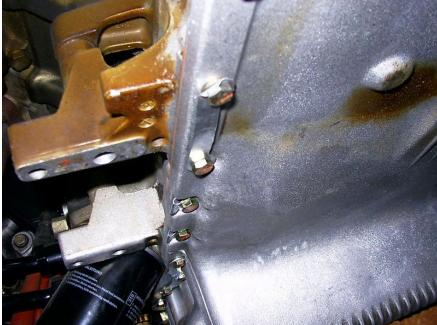
Instead of applying a torque wrench to the pan bolts, I tightened them by counting the number of fractional turns. I used a grease pencil to mark the bolt heads where tightened at the finger tight position, then tightened all bolts to  $\frac{1}{2}$  turn, in  $\frac{1}{8}$  turn increments, working my way around the pan.
