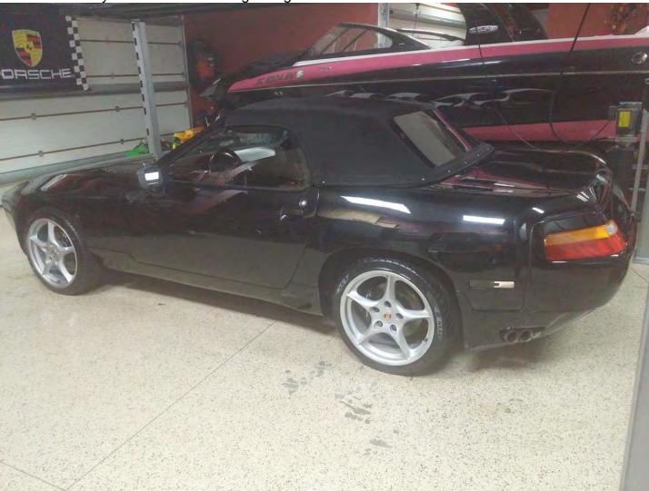
FRONT 225/40 ZR18 mounted on 8Jx18 ET 50 wheel REAR 285/30 R18 mounted on a 10Jx18 ET65 wheel
