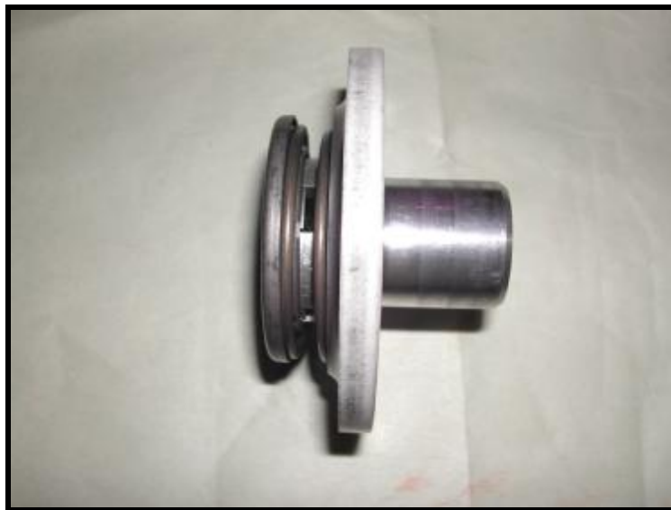
B2 Brake Band Piston Assembly with a view of retaining washer, spring, "T" plastic seal ring and OD of piston cylinder where lip seal seals
