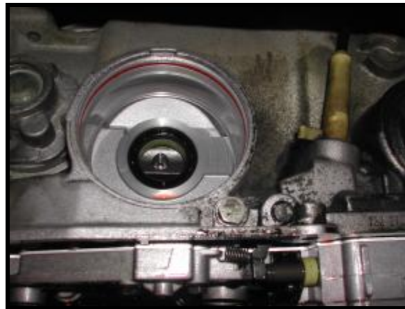
B2 Piston aperture showing black lip seal behind which is located the plastic guide bush. The location of the thrust pin into the brake band is also visible in the centre of the hole. Also visible is the cover O-ring seal (red)
