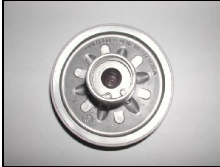
B2 Brake Band Piston Assembly With a view of thimble piece and retaining circlip
