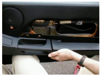
6. Once all of those bolts are out, you can pull the armrest off. It should just <u>lift right up</u>. This is on the passenger's side panel,
