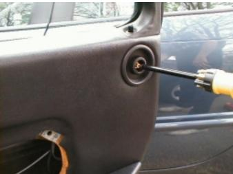
This will reveal a <u>screw</u> which holds the knob in. Remove the screw, then pull the knob straight off. Next the knob backing needs to be removed.
