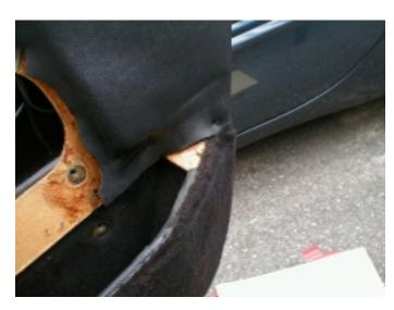
7. Then remove the <u>screw</u> at the rear of the panel (already removed in photo), at the base of where the armrest sat. There may also be another screw somewhere along the bottom of the door panel (I seem to recall one), but if there is, it is missing in my panel. Before proceeding to the next step just look around and make sure there aren't any other screws in the carpeted portion of the panel.
