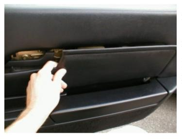
3. Now remove the door panel <u>insert</u>. It's held in at the top by white push-in clips, as well as being pushed down over the armrest. So first pry the upper rear portion away from the panel (the clips are both on the tip, one at the rear, one in the middle). Once both clips are out, then pull the insert upwards. In the photo, the clips have been pulled out of the panel (they should stay in the insert), and it is about to be pulled up.
