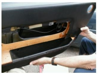
So once the clips are all out, you should lift it upwards, and towards the front of the car to remove it.
