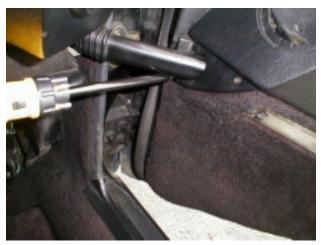
1. Remove the two screws holding in the <u>triangular piece</u> at the front of the door, where the wires enter. One screw is easy to see in the photo, the other is hidden, but the screwdriver is pointing at it. Once the screws are out, pull the triangular piece down a little (it wedges up under the armrest), and then back, like this.
