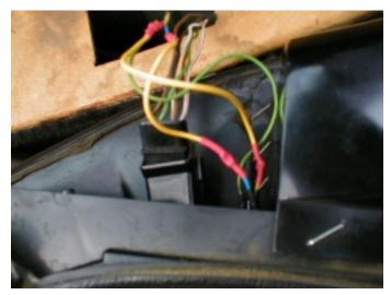
but on the driver's side panel when you remove the armrest you should just tilt it towards you some, exposing the <u>wires</u> on the underside of the power mirror switch (and seat position memory switch if you have it - I don't). Just unplug the wires. Make sure you keep track of which wires connect where on the crossover switch in front of the power mirror switch.
