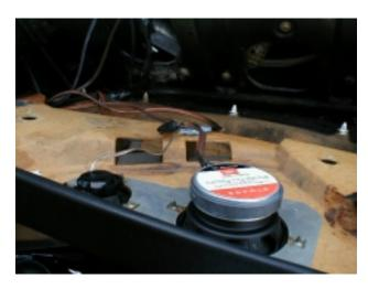
9. To pull the panel off the door, you need to pull the black plastic wire holder tube through the hole in the front of the panel.
