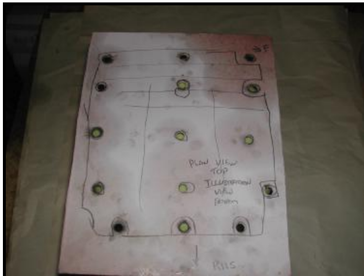
Valve Body Template to hold set bolts
