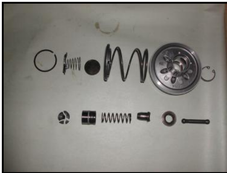
B2 Piston Assembly damage
