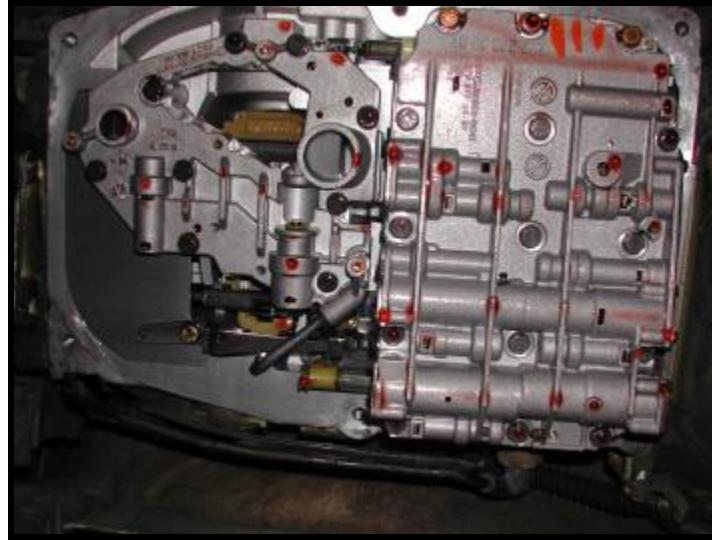
View of internals of AT with Pan and Filter Removed. On lower LHS space between centre is the oil pipe, detent quadrant leaf spring and Range (Gear) Selection Valve with Slide Head can be seen
