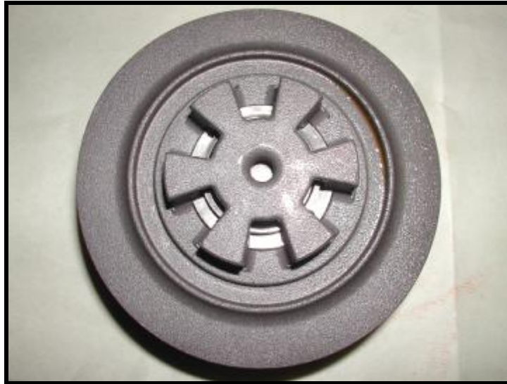
B2 Piston Old model Piston Assembly appears to be cast iron
