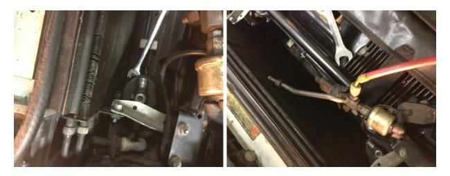
The filter dryer is 17mm connections if I recall correctly and the last connection on the driver side of the condenser requires two (2) 22mm.
