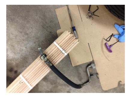
After I got all the O-rings replaced and everything put back I started at the front of the car changing out the filter/dryer. Needed a 19mm & 17mm to take the connection from condenser to the vertical pipe.
