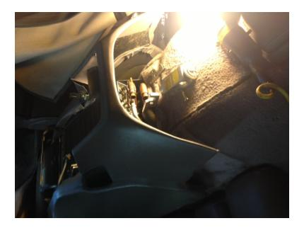
You don't have to remove the rear console in its entirety, just enough to get access to the expansion valve bolts. The T handle hex worked well here.
