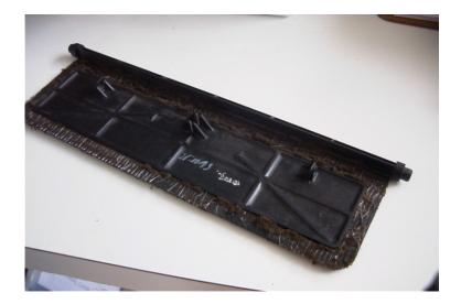
A special cut allows the flapper to be removed from the housing it lives in. I cut it so that the shaft of the plate does snap back into its location. The cut out piece only has to prevent the plate from lifting back out when in operation
