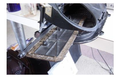
New Seals on both sides of the flapper valve installed prior to its return to its housing
