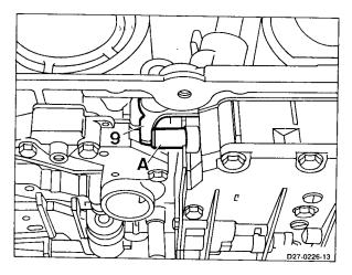
**Note:** The range selector lever (10) must engage in the follower (arrow) of the detent plate.
