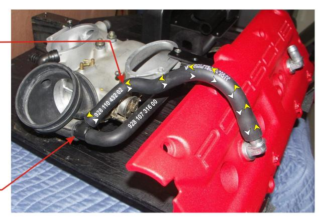
The PS rear elbow has an internal restricting orifice of 6mm. The PS front elbows (11.5mm) doesn't have a restricting orifice.
