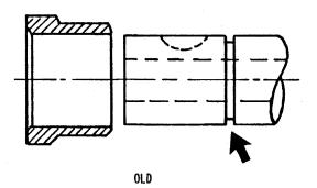
New-type camshafts no longer have groove (arrow).
