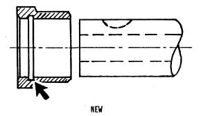
O-ring has been moved from camshafts to spacers (arrow).
