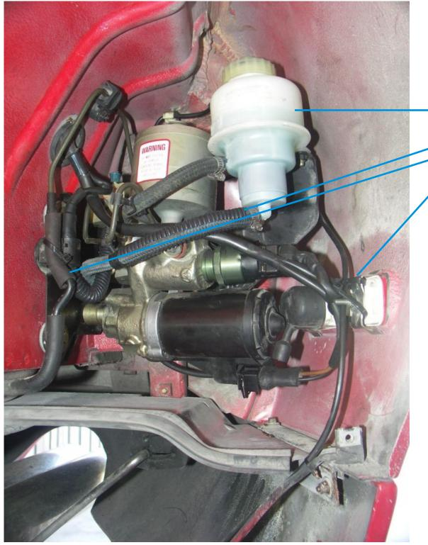
New reservoir system bled and flushed with fresh new fluid.
