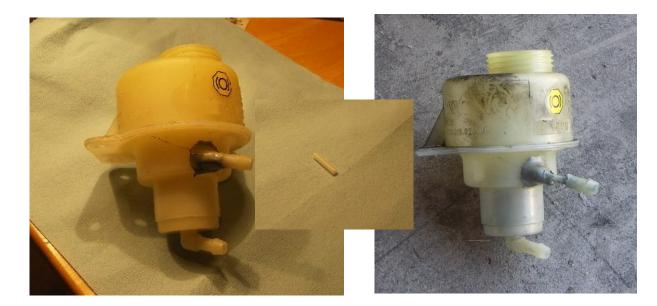
Early 2009 I had to make an emergency repair to my PSD reservoir return inlet pipe when I had removed it from the PSD unit it broke in an attempt to clean out the (noneremovable) internal filter as seen in the picture.
