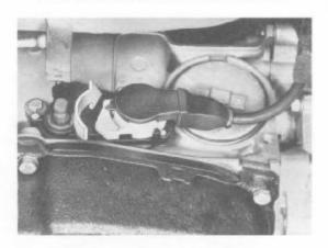
Pry off plug carefully with two screwdrivers applied on cable outlet and bar.
