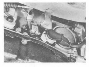
Remove bolt for range selector lever and pull off lever.
