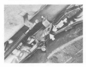
Unlock plug by turning white plastic ring (arrow) upwards in direction of arrow.
