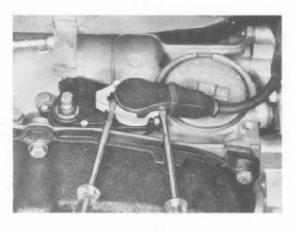
Remove switch mounting screws and take off switch.
