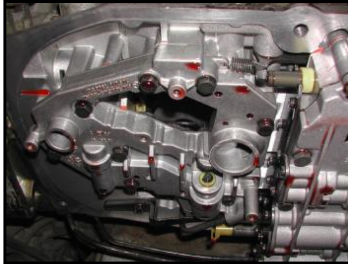
Lower Cover showing Controlled Pressure Control Valve Piston and Lever in the top RHS foreground with spring loaded actuating lever, Range (Gear) Selector Valve in the lower RHS background with its plastic slide that fits on pin of the detent quadrant and the suction and delivery orifices from the oil filter
