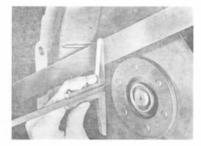
Install shim having thickness X (in example 5.3 mm).
