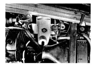
2. Move hydraulic unit into brackets from wheel side and insert two mounting bolts (position of mount as described in point 1).
