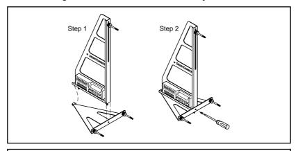
**Note:** 1. The SmartCamber tool will have to be recalibrated if the Hands Free adapter is removed or installed or if the tool is dropped. It should be checked periodically for calibration.
