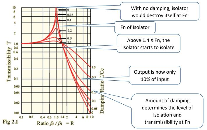
The curve above also shows the impact of damping. An isolator with no damping (damping ratio of zero) will wildly resonate and fail at its Fn, but will also significantly attenuate above Fn (attenuation actually starts at Fn X 1.4). As the curves show, if you increase damping, you reduce the transmissibility at Fn, but also reduce the amount of attenuation above Fn. Thus, specifying the amount damping becomes a balance of both resonance "craziness" and attenuation.
