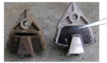
Filling in void makes isolator too stiff, not allowing for displacement
