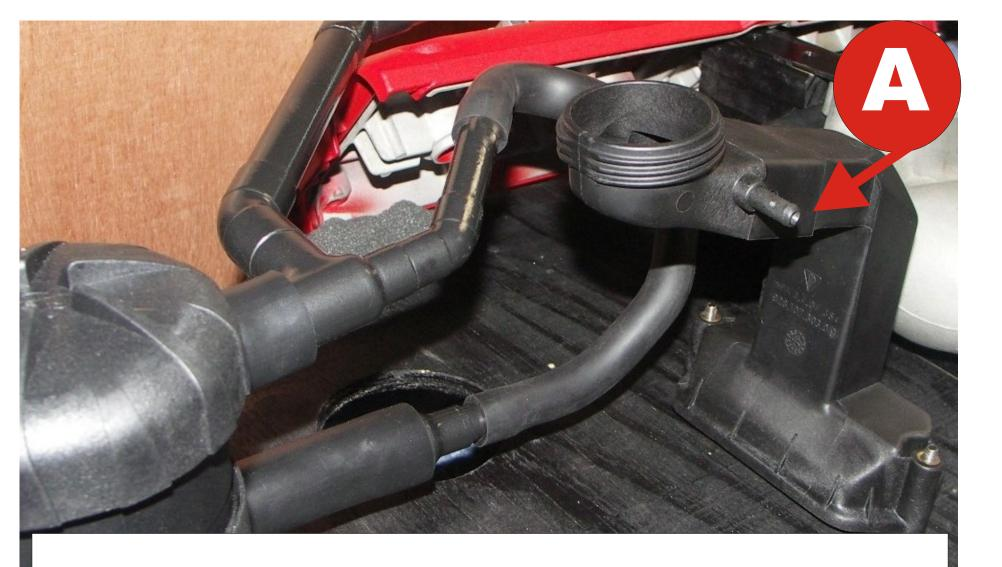
OFN Oil Filler Neck - The DS outlet (A) has an ID of 2.5mm and the connecting hose run to a connection on the throttle body on the GTS cars the factory has provided a "T" test port this the best place to check "manifold" Hg while the engine is running.
