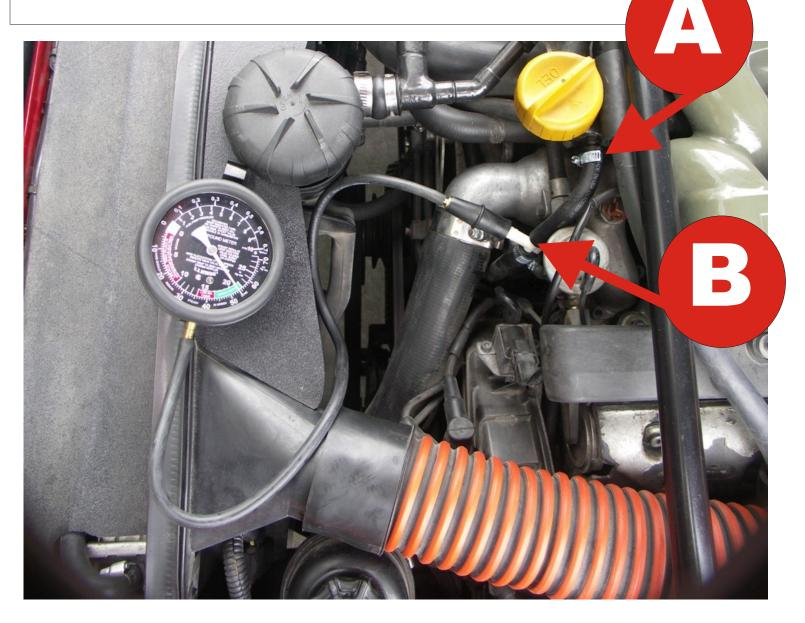
By connecting the OFN - DS 2.5mm orifice hose to the "T" that runs to the throttle body connection the VTG registers 1HG less versus the 2.5mm orifice being capped off.
