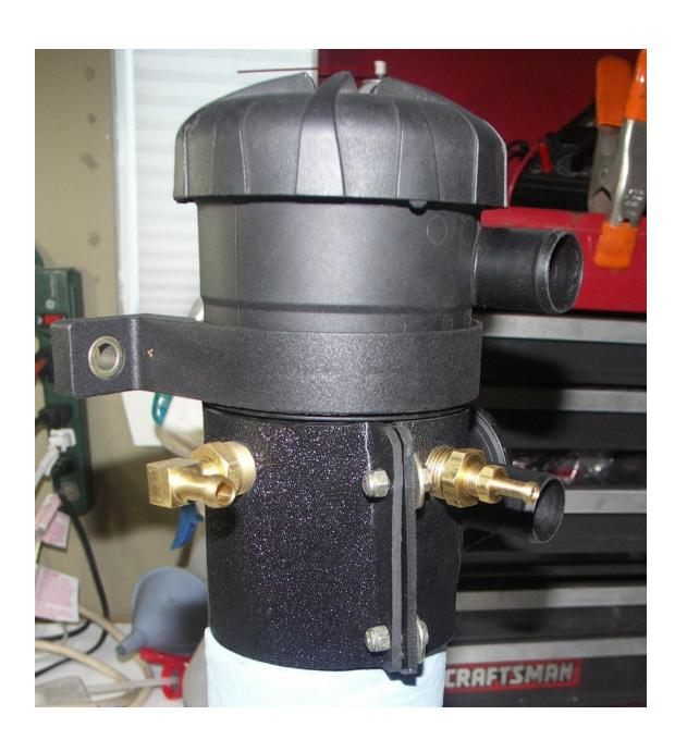
ABS base plate shaped into cylinder for the lower section of the Provent to increase wall thickness and placement of fittings.
