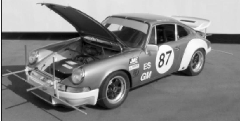
SmartStrings alignment kit. We now have what we believe to be the best and most universal way to quickly perform accurate four-wheel alignments on virtually any car anywhere.
