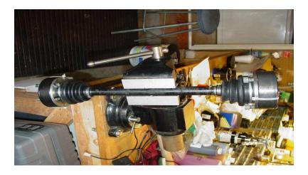
CV kit PN 928 332 924 01 contains boot PN 928 332 293 02 and fits new type shaft (one welded end, one bolted end) wheel and transaxle side flange as pictured. Flange has groove and boot has raised area on inner lip. Flange design is same on both the bolted and welded end. Each shaft requires 2 gaskets (1 between flange and bearing unit and 1 between bearing unit and wheel / transaxle mount).
