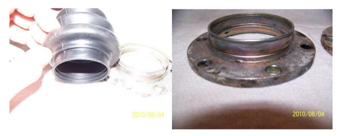
Boot large end opening stretches enough to fit over flange.
