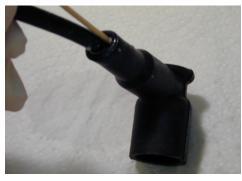
Move probe around the perimeter of the old wire, which will internally lubricate the boot and the wire.
