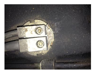
There are two (2) connections under the car towards the front. In my car they were just above the rear splash shield or the shield under the catalytic converters. I think they were 19mm & 17mm and 17mm & 14mm. After you replace the O-rings you can go back and install the bigger pipe in the previous one.
