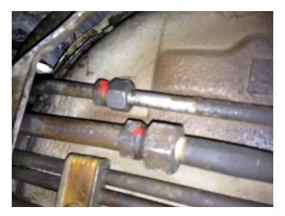
Now it is time to tackle the compressor. I just removed the four (4) bolts holding the compressor and wrestled it down. From the PET I was expecting more O-rings under the plate, but mine did not have any, so I could have replaced the hose O-rings with the compressor in place without removing the compressor entirely. The top plate of the compressor has a squarish type of gasket / O-ring. IF YOU REMOVE THE COMPRESSOR, BE CAREFUL OF THE ELECTRICAL CONNECTION.
