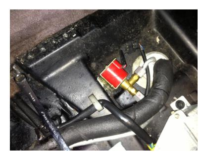
After that I tackled the rear AC expansion valve. I tried doing it without fully removing the rear console and it did not work.
