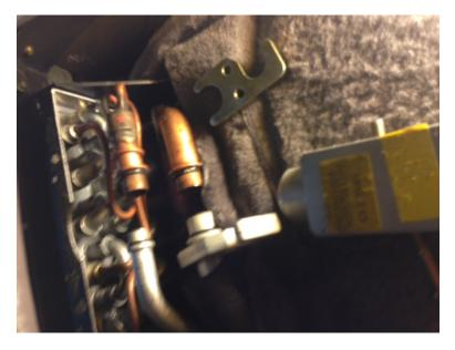
I then lifted the car up and started on the connection from under the car for the rear AC. It has two (2) 5mm bolts. After you remove the bolts the pipes can be pushed down. You can install the smaller pipe, but do not install the bigger pipe as yet.
