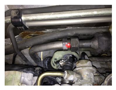
The next one I did was the solenoid under the passenger seat. YES, the seat has to come out. It took a 17mm & 14mm open end wrench. Be very careful as the aluminum lines are very fragile and they will twist when you try and overtigyhten them. In the picture you can see the top one starting to twist.
