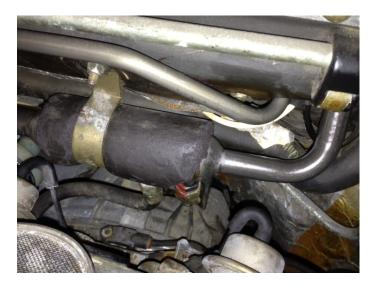
The other side needed a 32mm and a 27mm open ended wrench to undo the connection. The fuel cooler has to be able to be pushed towards the right to change this O-ring so after this is complete you can go back to the expansion valve and complete it.
