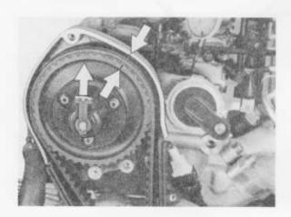
Note: Distributor rotor pointing upward.
