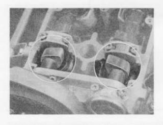
TDC mark with engine removed from car.
