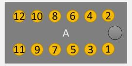
\*Motor potentiometer readings are approximate and based on test readings which can vary +/-50 $\Omega$  or more based on linkage adjustment, temps, etc. Ohms also can be checked across pins A5 and B8 (the other side of the FOOTWELL pot) which should show the same resistance range moving in the opposite direction relative to the position of the motor.
