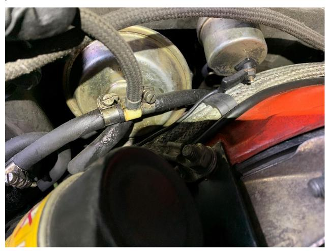
Electrical connection to the smaller (on the rear of the stock recirculation valve body) boost pressure sensor – I believe this one is for over-boost sensing the larger one on the front is for the boost pressure gauge.
