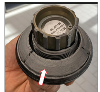
Figure 5 Application of Grease to Centerlock Cone
