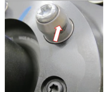
Figure 3 Material Transfer on Drive Peg
