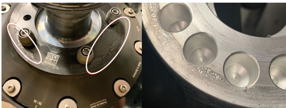
Figure 2 Material Transfer to Brake Disc Bell (Left) from Wheel (Right)
